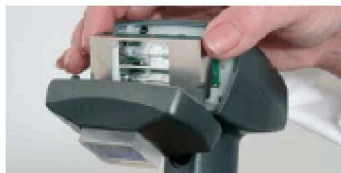
The handset hinges open to allow access to the lamp unit.
